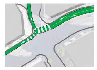
Transition at Minor/Melrose between the Pike Pine Renaissance bike lanes and each alignment option on Pike.
